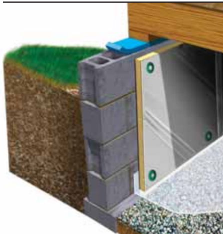
The non-vented crawl space system uses rigid foam insulation on the foundation wall interior to reduce the potential for condensation and related moisture problems.
